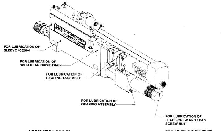
LUBRICATION POINTS (GREASE FITTING LOCATIONS)
